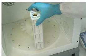
5. Place segment into the rotor plate
