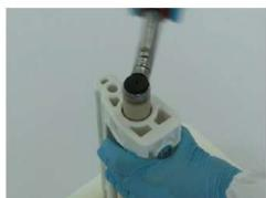
4. Tighten with torque wrench
